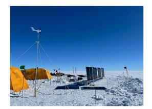
Power from the system runs a multitude of sensors and electrical measurement equipment, including the Automatic Surface Flux Station (ASFS), Ground Penetrating Radar (GPR), Micro Rain Radar (MRR), Microwave Radiometer (MWR), Ice Mass Balance (IMB), Open GNSS Research Equipment (OGRE), Portable Optical Particle Spectrometer (POPS), as well as other electronics.
